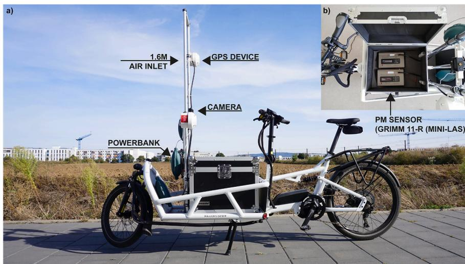
Fig. 2. Photographs of the electro cargo bike with GPS device, powerbank, camera (a) and the box containing PM sensors, GRIMM 11-R PM sensors (b).
