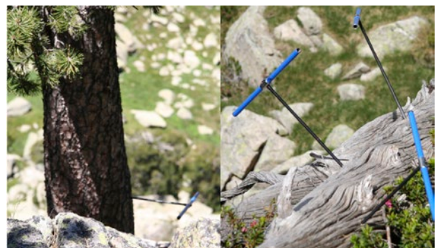
Fig. 1. Increment borers used to sample 5 mm diameter cores from living (left) and dead (right) Pinus uncinata near the timberline in the Spanish Pyrenees.
